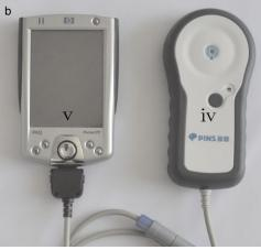
**Figure 1.** Photo of PINS device. a. implantable parts including (i) implantable pulse generator (IPG), (ii) extension, and (iii) lead; b. telemetry/programming parts including (iv) controller and (v) personal digital assistant (PDA).
